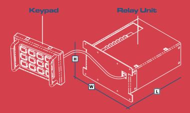
The InControl 12 power control module which consists of a relay unit and a 12-key keypad. The keypad can be remotely mounted or installed on the relay unit. Each independantly configurable key controls a relay which, in turn, applies power to an output device. The InControl 12 can control up to 12 output devices. It uses high current, automotive grade relays to ensure reliable operation and minimize maintenance.
